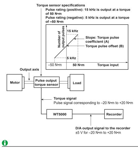
The pulse input range setting applies to input signals whose type has been set to pulse. For input signals whose type has been set to analog, there is no need to configure this setting.
