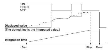
• If you stop integration while the display is held, the displayed and transmitted values do not change. When you release the hold function (turn it off) or make a single measurement, the integration result at the point when integration was stopped is displayed and transmitted.
