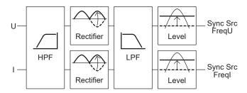
• Turning the Frequency Filter (HPF) On and Off (Freq Filter) Turn the frequency filter (HPF) on or off.
