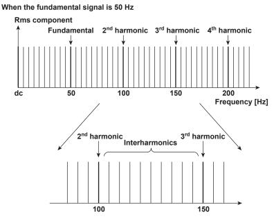
If the input signal is 60 Hz, 12 periods of the waveform are divided in 5-Hz resolution. Thus, the section between each harmonic order is divided into 12 sections.
