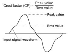
On this instrument, the crest factor is the ratio of the maximum applicable peak value to the measurement range.
