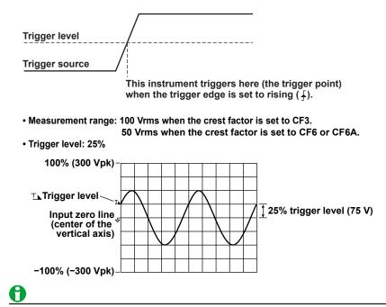
If you do not set the trigger level properly, the waveform display start point (the signal level on the left edge of the screen) may be unstable, or waveforms may not appear.
