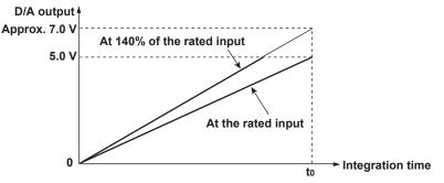
t0: The rated time of integrated D/A output in manual integration mode. The timer time in normal or continuous integration mode.
