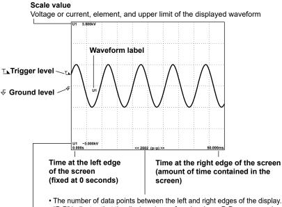
• "P-P" indicates that the displayed waveform has been P-P compressed.
