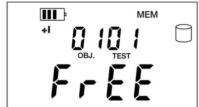
The instrument proposes the first free location in memory. If it is acceptable, execute a long press on the MEM key. To change the number of the test or of the object, use
