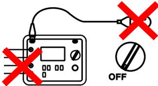
Use a soft cloth, dampened with soapy water. Rinse with a damp cloth and dry rapidly with a dry cloth or forced air. Do not use alcohol, solvents, or hydrocarbons.
