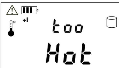
If a measurement in the 10 A range lasts several minutes, it causes internal overheating, making all measurements impossible. It is then necessary to wait for the instrument to cool before resuming the measurements.
