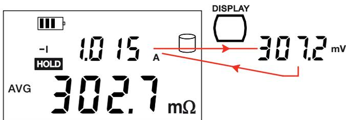
To display the voltage on the terminals of the resistance instead of the measurement current, press the DISPLAY key.
