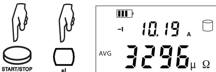
Reverse the direction of the current by pressing the ±I key and the instrument displays the average:
