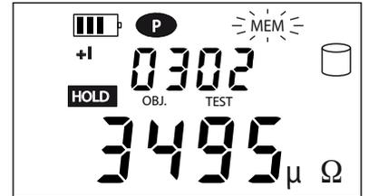
At each new measurement, the test number is incremented and the measurement is recorded.
