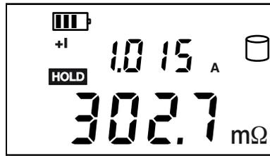
If the measurement is stopped by the disconnection of a clip, simply connecting it to another object starts another measurement, with no need to press the START/STOP key.
