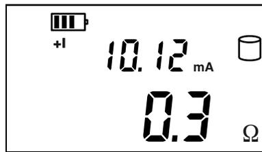
If the measurement is too low, turn the switch to the next lower range and restart the measurement. Continue until the display shows at least 3 digits.
