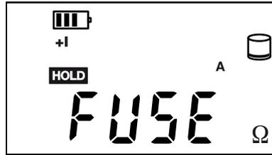
If a voltage greater than 20 V is applied between terminals C1 and C2, the fuse on the front panel of the instrument will blow and must be replaced (see §7.2).
