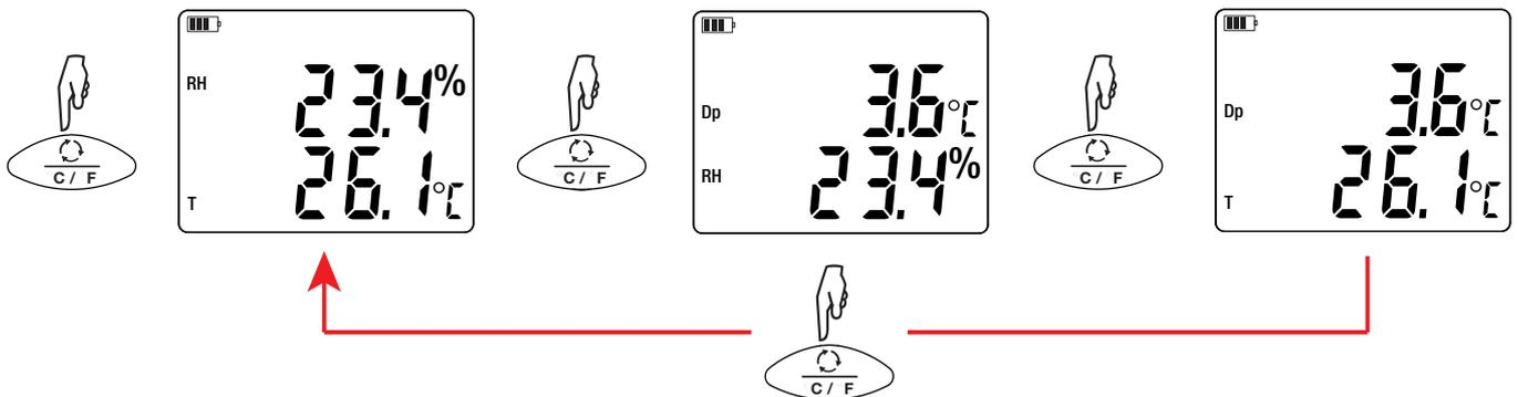
The last display selected is saved when the instrument is switched off.
