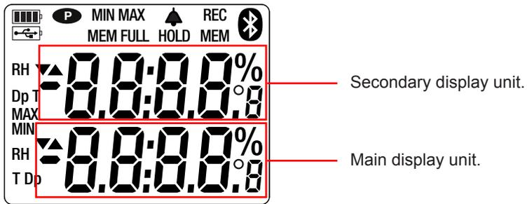
When the measurement exceeds the limits (positive or negative), the instrument displays OL.
