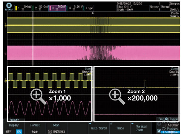
Detailed waveform measured for 20 seconds are shown in 20 milliseconds and 100 microseconds span.
