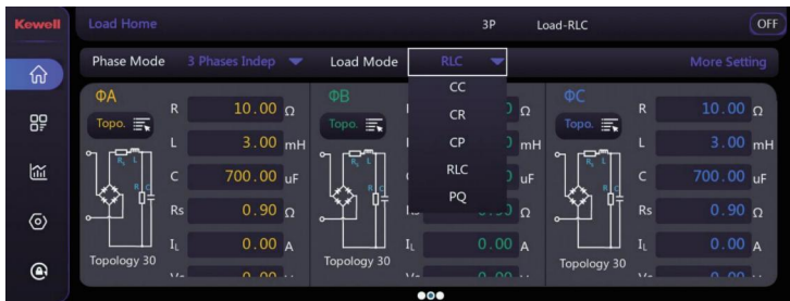
Rectifier topology in RLC mode
