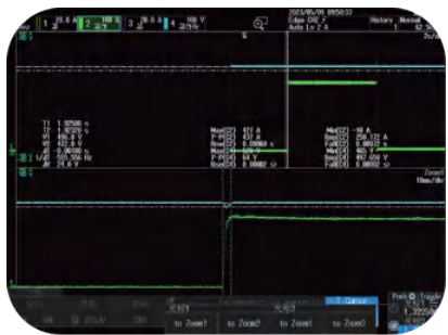
Sudden loading at 500V, voltage fluctuation: 24V@400A
